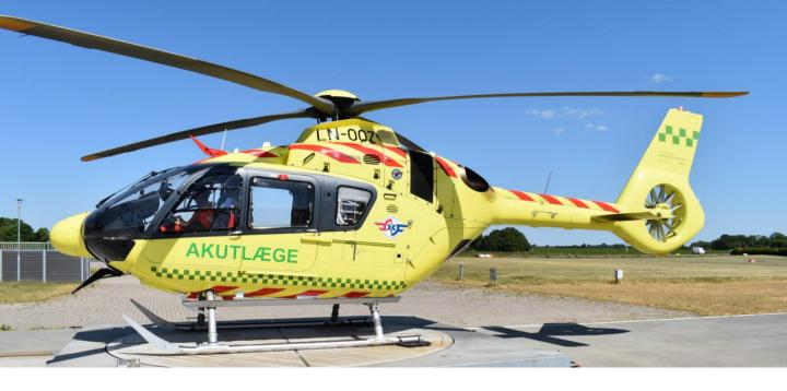
3x EC135P3 in HEMS configuration SP/DP IFR NVIS Certified
